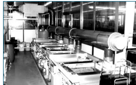
Abwasserlose Brünieranlage Bronzing installation without waste water Installation de bronzage sans eaux usées
